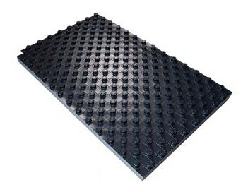
Thermoformed insulation panel R979G for radiant floor systems. Consisting of expanded polystyrene foam (EPS) with graphite and black thermoformed polystyrene protection layer. The combination of these two elements and their intrinsic characteristics provide a panel with a resistance to trampling deformation much greater than traditional thermoformed insulation panels.
