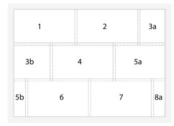
After fitting edge strip K369A on the walls (the insulation that prevents heat bridges and allows minimum dilations of the floor), lay and connect the panels making sure the subsequent rows follow an offset pattern.
